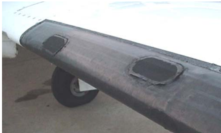
De-Icing Boot with Patch Repairs
