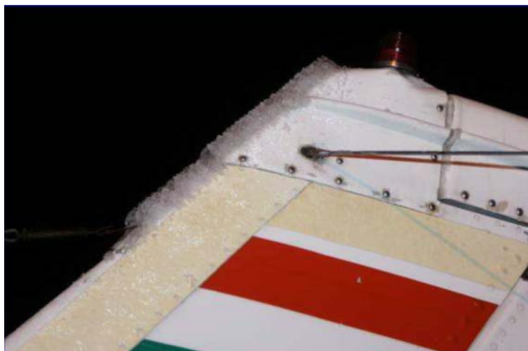
Ice on low radius of curvature aerofoils
